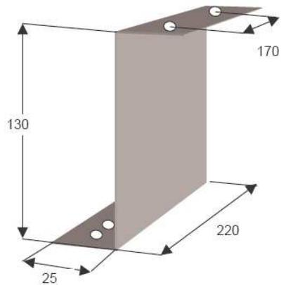
The cyclones are hanged against a vertical surface by means of two stainless steel support clamps and two clamping rings made of also stainless steel.
